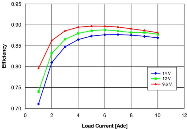
**Fig. 1.2V.3:** Efficiency vs. load current and input voltage for V<sub>out</sub> = 1.2 V converter mounted vertically with air flowing at a rate of 200 LFM (1 m/s) and T<sub>a</sub> = 25 °C.
