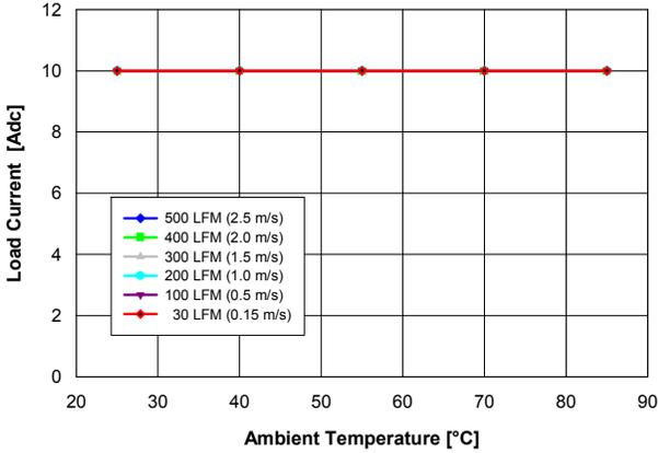
**Fig. 1.2V.1:** Available load current vs. ambient temperature and airflow rates for V<sub>out</sub> = 1.2 V converter mounted vertically with V<sub>in</sub> = 12 V, and maximum MOSFET temperature ≤ 110 °C.
