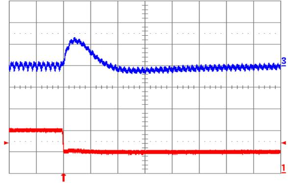
**Fig. 2.5V.8:** Output voltage response for  $V_{out} = 2.5$  V to negative load current step change from 10 A to 5 A with slew rate of  $-5 \text{ A}/\mu\text{s}$  at  $V_{in} = 12$  V. Top trace: output voltage (100 mV/div.); Bottom trace: load current (5 A/div.).  $C_o = 100 \mu\text{F}$  ceramic. Time scale: 20  $\mu\text{s}$ /div.
