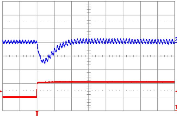
**Fig. 5.0V.7:** Output voltage response for  $V_{out} = 5.0$  V to positive load current step change from 5 A to 10 A with slew rate of 5 A/ $\mu\text{s}$  at  $V_{in} = 12$  V. Top trace: output voltage (100 mV/div.); Bottom trace: load current (5 A/div.).  $C_o = 100 \mu\text{F}$  ceramic. Time scale: 20  $\mu\text{s}$ /div.
