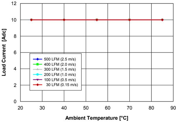
**Fig. 2.5V.1:** Available load current vs. ambient temperature and airflow rates for  $V_{out} = 2.5$  V converter mounted vertically with  $V_{in} = 12$  V, and maximum MOSFET temperature  $\leq 110$  °C.
