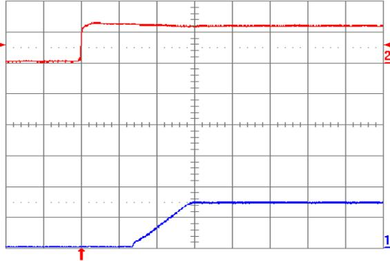
**Fig. 1.5V.5:** Turn-on transient for  $V_{out} = 1.5$  V with application of  $V_{in}$  at full rated load current (resistive) and  $100 \mu\text{F}$  external capacitance at  $V_{in} = 12$  V. Top trace:  $V_{in}$  (10 V/div.); Bottom trace: output voltage (1 V/div.); Time scale: 2 ms/div.
