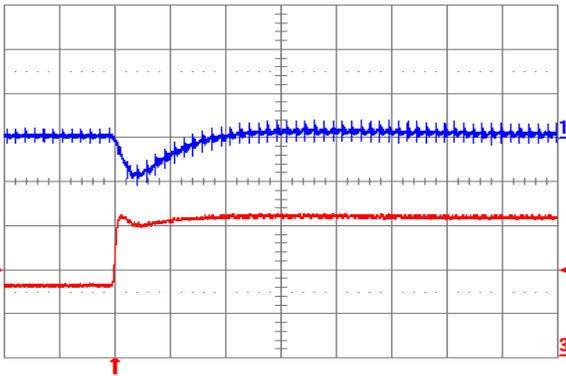
**Fig. 0.7525V.7:** Output voltage response for  $V_{out} = 0.7525$  V to positive load current step change from 5 A to 10 A with slew rate of  $5 \text{ A}/\mu\text{s}$  at  $V_{in} = 12$  V. Top trace: output voltage (100 mV/div.); Bottom trace: load current (5 A/div.).  $C_o = 100 \mu\text{F}$  ceramic. Time scale: 20  $\mu\text{s}$ /div.
