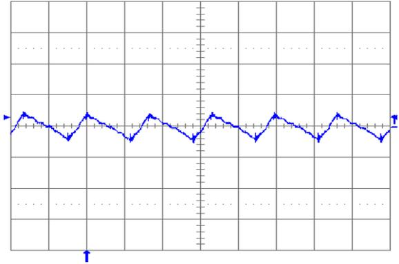
**Fig. 3.3V.6:** Output voltage ripple (20 mV/div.) at full rated load current into a resistive load with external capacitance  $100 \mu\text{F}$  ceramic +  $1 \mu\text{F}$  ceramic, and  $V_{in} = 12$  V for  $V_{out} = 3.3$  V. Time scale: 2  $\mu\text{s}$ /div.
