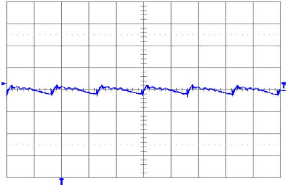
**Fig. 1.2V.6:** Output voltage ripple (20 mV/div.) at full rated load current into a resistive load with external capacitance  $100 \mu\text{F}$  ceramic +  $1 \mu\text{F}$  ceramic, and  $V_{in} = 12$  V for  $V_{out} = 1.2$  V. Time scale: 2  $\mu\text{s}$ /div.
