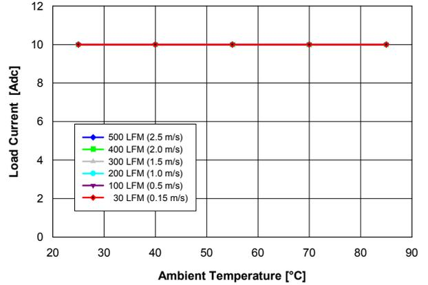
**Fig. 1.0V.2:** Available load current vs. ambient temperature and airflow rates for  $V_{out} = 1.0$  V converter mounted horizontally with  $V_{in} = 12$  V, and maximum MOSFET temperature  $\leq 110$  °C.
