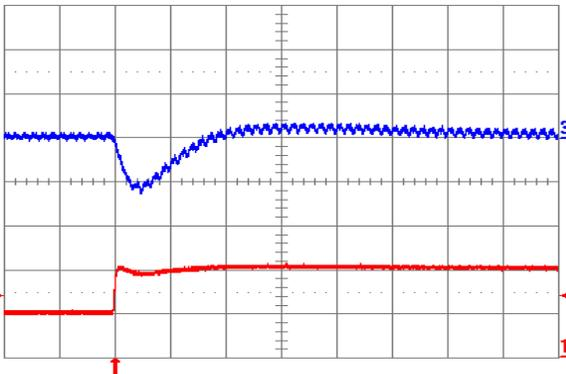
**Fig. 1.2V.7:** Output voltage response for  $V_{out} = 1.2$  V to positive load current step change from 5 A to 10 A with slew rate of 5 A/ $\mu\text{s}$  at  $V_{in} = 12$  V. Top trace: output voltage (100 mV/div.); Bottom trace: load current (5 A/div.).  $C_o = 100 \mu\text{F}$  ceramic. Time scale: 20  $\mu\text{s}$ /div.
