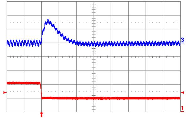
**Fig. 5.0V.8:** Output voltage response for  $V_{out} = 5.0$  V to negative load current step change from 10 A to 5 A with slew rate of -5 A/ $\mu\text{s}$  at  $V_{in} = 12$  V. Top trace: output voltage (100 mV/div.); Bottom trace: load current (5 A/div.).  $C_o = 100 \mu\text{F}$  ceramic. Time scale: 20  $\mu\text{s}$ /div.
