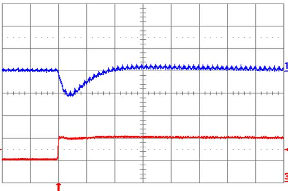
**Fig. 1.0V.7:** Output voltage response for  $V_{out} = 1.0$  V to positive load current step change from 5 A to 10 A with slew rate of  $5 \text{ A}/\mu\text{s}$  at  $V_{in} = 12$  V. Top trace: output voltage (100 mV/div.); Bottom trace: load current (5 A/div.).  $C_o = 100 \mu\text{F}$  ceramic. Time scale: 20  $\mu\text{s}$ /div.
