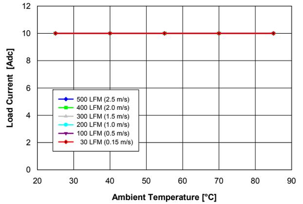
**Fig. 3.3V.2:** Available load current vs. ambient temperature and airflow rates for  $V_{out} = 3.3$  V converter mounted horizontally with  $V_{in} = 12$  V, and maximum MOSFET temperature  $\leq 110$  °C.
