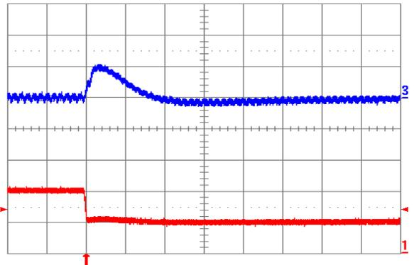
**Fig. 1.2V.8:** Output voltage response for  $V_{out} = 1.2$  V to negative load current step change from 10 A to 5 A with slew rate of -5 A/ $\mu\text{s}$  at  $V_{in} = 12$  V. Top trace: output voltage (100 mV/div.); Bottom trace: load current (5 A/div.).  $C_o = 100 \mu\text{F}$  ceramic. Time scale: 20  $\mu\text{s}$ /div.
