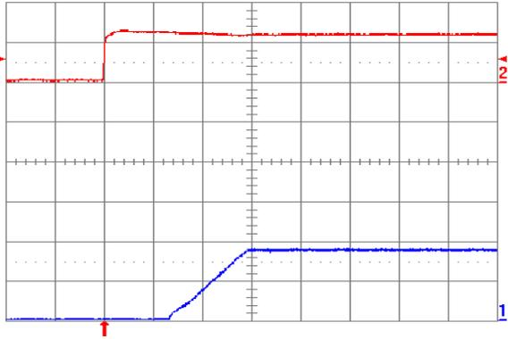
**Fig. 1.8V.5:** Turn-on transient for  $V_{out} = 1.8$  V with application of  $V_{in}$  at full rated load current (resistive) and  $100 \mu\text{F}$  external capacitance at  $V_{in} = 12$  V. Top trace:  $V_{in}$  (10 V/div.); Bottom trace: output voltage (1 V/div.); Time scale: 2 ms/div.
