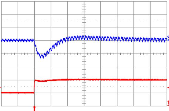
**Fig. 2.5V.7:** Output voltage response for  $V_{out} = 2.5$  V to positive load current step change from 5 A to 10 A with slew rate of  $5 \text{ A}/\mu\text{s}$  at  $V_{in} = 12$  V. Top trace: output voltage (100 mV/div.); Bottom trace: load current (5 A/div.).  $C_o = 100 \mu\text{F}$  ceramic. Time scale: 20  $\mu\text{s}$ /div.
