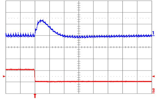
**Fig. 2.0V.8:** Output voltage response for  $V_{out} = 2.0$  V to negative load current step change from 10 A to 5 A with slew rate of  $-5 \text{ A}/\mu\text{s}$  at  $V_{in} = 12$  V. Top trace: output voltage (100 mV/div.); Bottom trace: load current (5 A/div.).  $C_o = 100 \mu\text{F}$  ceramic. Time scale: 20  $\mu\text{s}$ /div.
