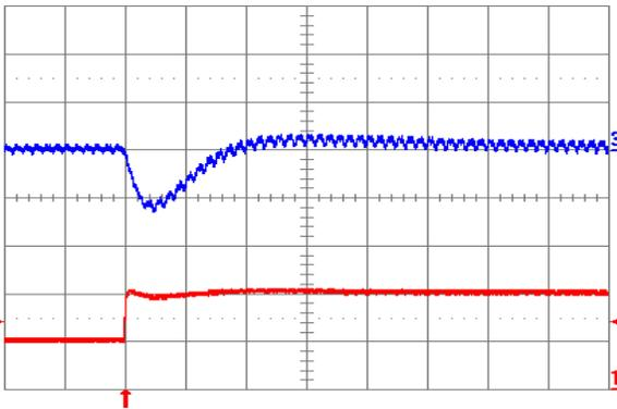
**Fig. 1.5V.7:** Output voltage response for  $V_{out} = 1.5$  V to positive load current step change from 5 A to 10 A with slew rate of  $5 \text{ A}/\mu\text{s}$  at  $V_{in} = 12$  V. Top trace: output voltage (100 mV/div.); Bottom trace: load current (2 A/div.).  $C_o = 100 \mu\text{F}$  ceramic. Time scale: 20  $\mu\text{s}$ /div.
