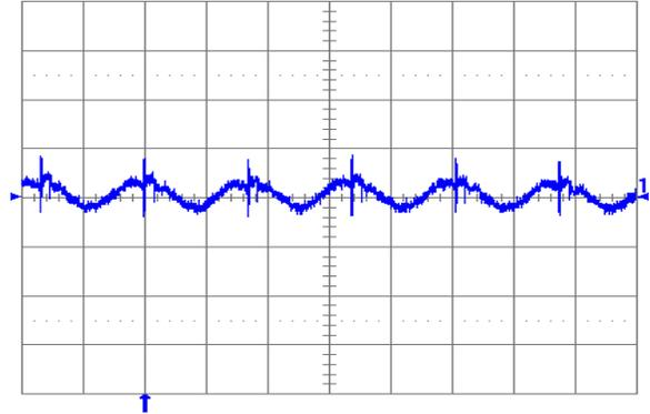
**Fig. 0.7525V.6:** Output voltage ripple (20 mV/div.) at full rated load current into a resistive load with external capacitance  $100 \mu\text{F}$  ceramic +  $1 \mu\text{F}$  ceramic, and  $V_{in} = 12$  V for  $V_{out} = 0.7525$  V. Time scale: 2  $\mu\text{s}$ /div.
