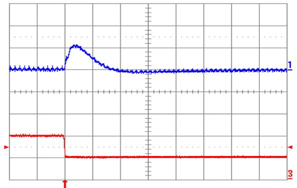
**Fig. 1.0V.8:** Output voltage response for  $V_{out} = 1.0$  V to negative load current step change from 10 A to 5 A with slew rate of  $-5 \text{ A}/\mu\text{s}$  at  $V_{in} = 12$  V. Top trace: output voltage (100 mV/div.); Bottom trace: load current (5 A/div.).  $C_o = 100 \mu\text{F}$  ceramic. Time scale: 20  $\mu\text{s}$ /div.
