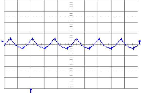
**Fig. 5.0V.6:** Output voltage ripple (20 mV/div.) at full rated load current into a resistive load with external capacitance  $100 \mu\text{F}$  ceramic +  $1 \mu\text{F}$  ceramic, and  $V_{in} = 12$  V for  $V_{out} = 5.0$  V. Time scale: 2  $\mu\text{s}$ /div.
