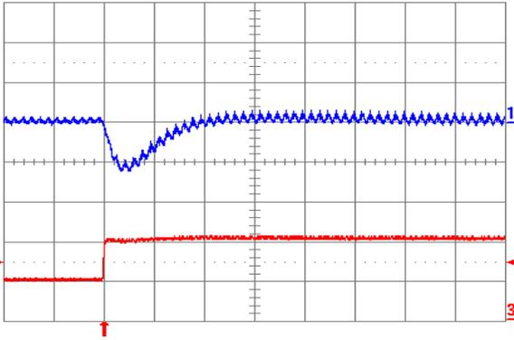
**Fig. 2.0V.7:** Output voltage response for  $V_{out} = 2.0$  V to positive load current step change from 5 A to 10 A with slew rate of  $5 \text{ A}/\mu\text{s}$  at  $V_{in} = 12$  V. Top trace: output voltage (100 mV/div.); Bottom trace: load current (5 A/div.).  $C_o = 100 \mu\text{F}$  ceramic. Time scale: 20  $\mu\text{s}$ /div.
