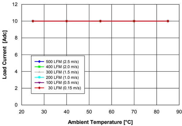
**Fig. 3.3V.1:** Available load current vs. ambient temperature and airflow rates for  $V_{out} = 3.3$  V converter mounted vertically with  $V_{in} = 12$  V, and maximum MOSFET temperature  $\leq 110$  °C.
