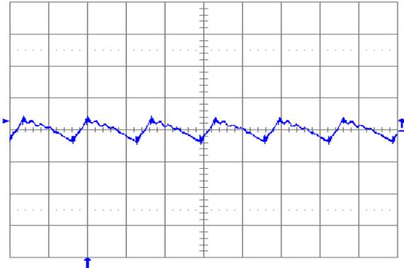
**Fig. 2.5V.6:** Output voltage ripple (20 mV/div.) at full rated load current into a resistive load with external capacitance  $100 \mu\text{F}$  ceramic +  $1 \mu\text{F}$  ceramic, and  $V_{in} = 12$  V for  $V_{out} = 2.5$  V. Time scale: 2  $\mu\text{s}$ /div.
