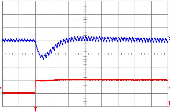
**Fig. 3.3V.7:** Output voltage response for  $V_{out} = 3.3$  V to positive load current step change from 5 A to 10 A with slew rate of  $5 \text{ A}/\mu\text{s}$  at  $V_{in} = 12$  V. Top trace: output voltage (100 mV/div.); Bottom trace: load current (5 A/div.).  $C_o = 100 \mu\text{F}$  ceramic. Time scale: 20  $\mu\text{s}$ /div.
