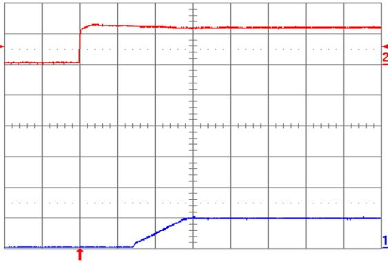
**Fig. 1.0V.5:** Turn-on transient for  $V_{out} = 1.0$  V with application of  $V_{in}$  at full rated load current (resistive) and  $100 \mu\text{F}$  external capacitance at  $V_{in} = 12$  V. Top trace:  $V_{in}$  (10 V/div.); Bottom trace: output voltage (1 V/div.); Time scale: 2 ms/div.
