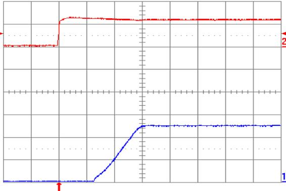
**Fig. 2.5V.5:** Turn-on transient for  $V_{out} = 2.5$  V with application of  $V_{in}$  at full rated load current (resistive) and  $47 \mu\text{F}$  external capacitance at  $V_{in} = 12$  V. Top trace:  $V_{in}$  (10 V/div.); Bottom trace: output voltage (1 V/div.); Time scale: 2 ms/div.
