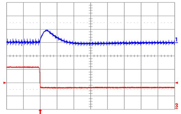
**Fig. 0.7525V.8:** Output voltage response for  $V_{out} = 0.7525$  V to negative load current step change from 10 A to 5 A with slew rate of  $-5 \text{ A}/\mu\text{s}$  at  $V_{in} = 12$  V. Top trace: output voltage (100 mV/div.); Bottom trace: load current (5 A/div.).  $C_o = 100 \mu\text{F}$  ceramic. Time scale: 20  $\mu\text{s}$ /div.
