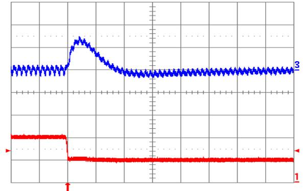
**Fig. 3.3V.8:** Output voltage response for  $V_{out} = 3.3$  V to negative load current step change from 10 A to 5 A with slew rate of  $-5 \text{ A}/\mu\text{s}$  at  $V_{in} = 12$  V. Top trace: output voltage 100 mV/div.; Bottom trace: load current (2 A/div.).  $C_o = 100 \mu\text{F}$  ceramic. Time scale: 20  $\mu\text{s}$ /div.
