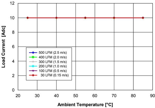
**Fig. 1.8V.1:** Available load current vs. ambient temperature and airflow rates for  $V_{out} = 1.8$  V converter mounted vertically with  $V_{in} = 12$  V, and maximum MOSFET temperature  $\leq 110$  °C.
