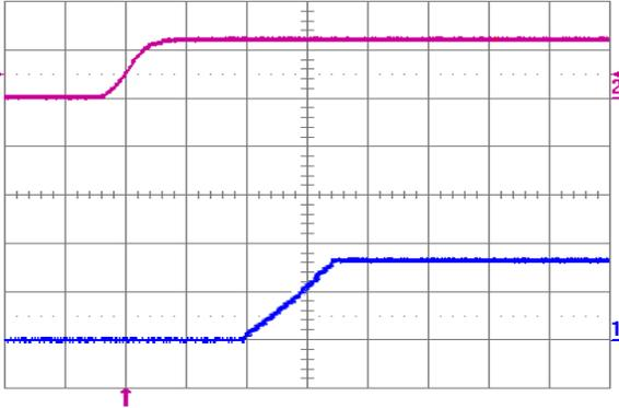
**Fig. 0.7525V.5:** Turn-on transient for  $V_{out} = 0.7525$  V with application of  $V_{in}$  at full rated load current (resistive) and  $100 \mu\text{F}$  external capacitance at  $V_{in} = 12$  V. Top trace:  $V_{in}$  (10 V/div.); Bottom trace: output voltage (0.5 V/div.); Time scale: 2 ms/div.
