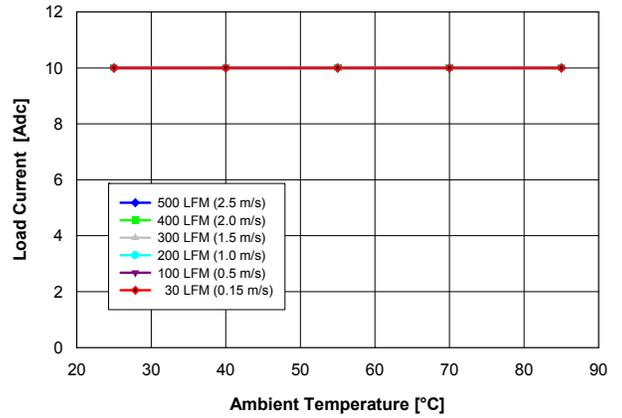
**Fig. 2.5V.2:** Available load current vs. ambient temperature and airflow rates for  $V_{out} = 2.5$  V converter mounted horizontally with  $V_{in} = 12$  V, and maximum MOSFET temperature  $\leq 110$  °C.
