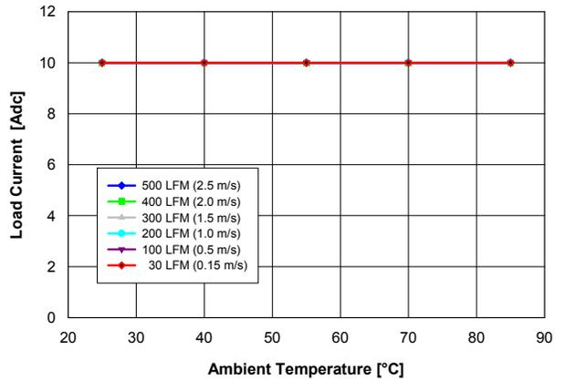
**Fig. 1.8V.2:** Available load current vs. ambient temperature and airflow rates for  $V_{out} = 1.8$  V converter mounted horizontally with  $V_{in} = 12$  V, and maximum MOSFET temperature  $\leq 110$  °C.
