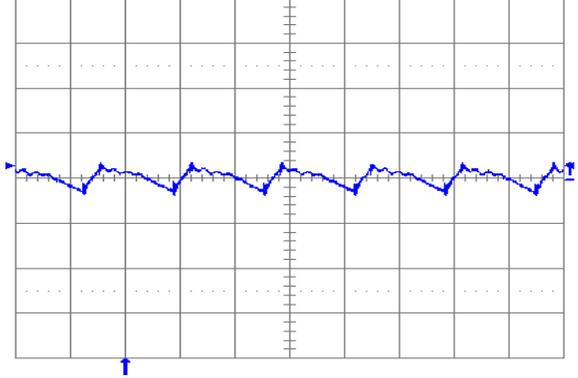
**Fig. 2.0V.6:** Output voltage ripple (20 mV/div.) at full rated load current into a resistive load with external capacitance  $100 \mu\text{F}$  ceramic +  $1 \mu\text{F}$  ceramic, and  $V_{in} = 12$  V for  $V_{out} = 2.0$  V. Time scale: 2  $\mu\text{s}$ /div.
