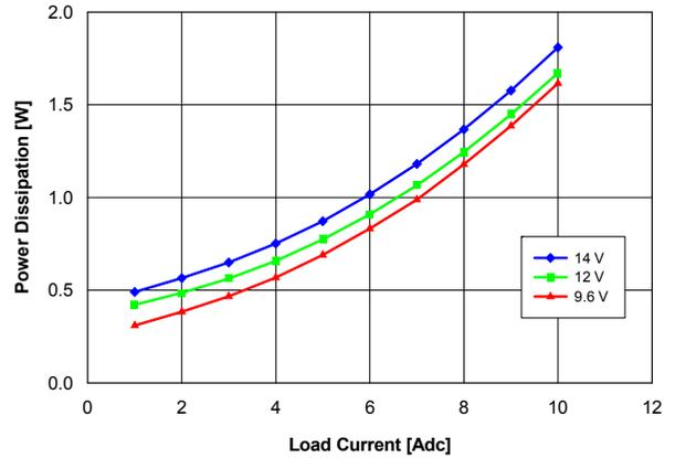
**Fig. 1.2V.4:** Power loss vs. load current and input voltage for V<sub>out</sub> = 1.2 V converter mounted vertically with air flowing at a rate of 200 LFM (1 m/s) and T<sub>a</sub> = 25 °C.
