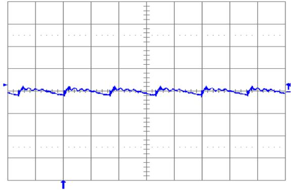
**Fig. 1.0V.6:** Output voltage ripple (20 mV/div.) at full rated load current into a resistive load with external capacitance  $100 \mu\text{F}$  ceramic +  $1 \mu\text{F}$  ceramic, and  $V_{in} = 12$  V for  $V_{out} = 1.0$  V. Time scale: 2  $\mu\text{s}$ /div.
