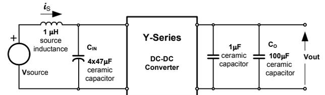
**Fig. E:** Test setup for measuring input reflected-ripple currents,  $i_s$  and output voltage ripple.
