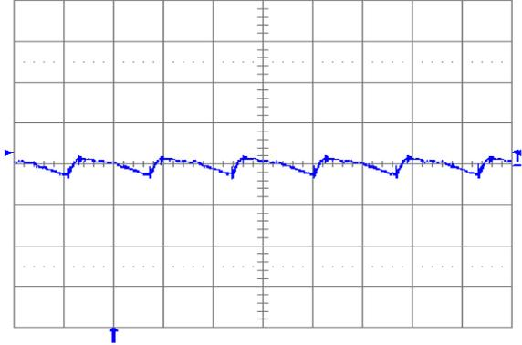
**Fig. 1.5V.6:** Output voltage ripple (20 mV/div.) at full rated load current into a resistive load with external capacitance  $100 \mu\text{F}$  ceramic +  $1 \mu\text{F}$  ceramic, and  $V_{in} = 12$  V for  $V_{out} = 1.5$  V. Time scale: 2  $\mu\text{s}$ /div.
